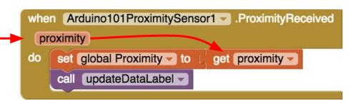
Your app should now be working! Connect your Arduino device using the MIT Al2 Companion (if you haven't already). Test it out by moving your hand closer and farther away from the sensor. If it is working, you should see the data label change.
