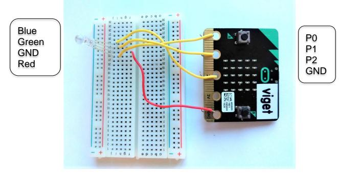
Bend the wire to U shape and hook on Micro:bit pins.
