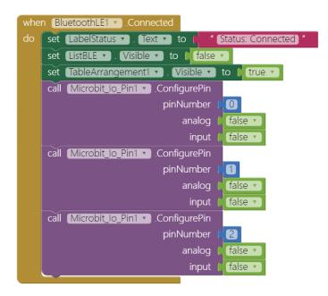
Let's get a look at **Microbit\_lo\_Pin.ConfigurePin** method. It has three parameters: **pinNumber (pin index)**, **analog** (true to analog, false to digital) and **input** (true to input, false to output).
